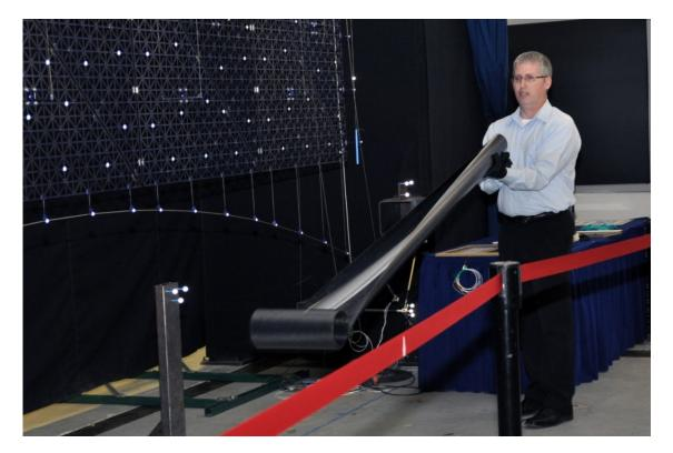
AFRL scientist Paul Hausgen demonstrates deploying the composite Roll-Out Solar Array slit-tube boom. The booms do not require external power but deploy under their own stored strain energy.
