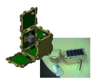
**CubeFlow -** A miniaturized SPA-U based modular system designed to be compliant with the popular CubeSat standard. Used to support simple space experiments and outreach.
