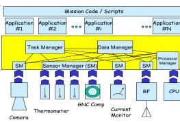
**SPA software -** The satellite data model handles the internal organization of data in the SPA approach. Electronic datasheets in hardware and software are used to cue the self-organization of systems.
