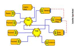
**SPA networks -** Components are plug-and-play objects that can be freely interconnected through hubs or routers that automatically distribute power, data and synchronization signals.
