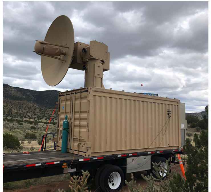
The Air Force Research Laboratory's Tactical High Power Operational Responder developed for airbase defense. Photo credit: AFRL Directed Energy Directorate
