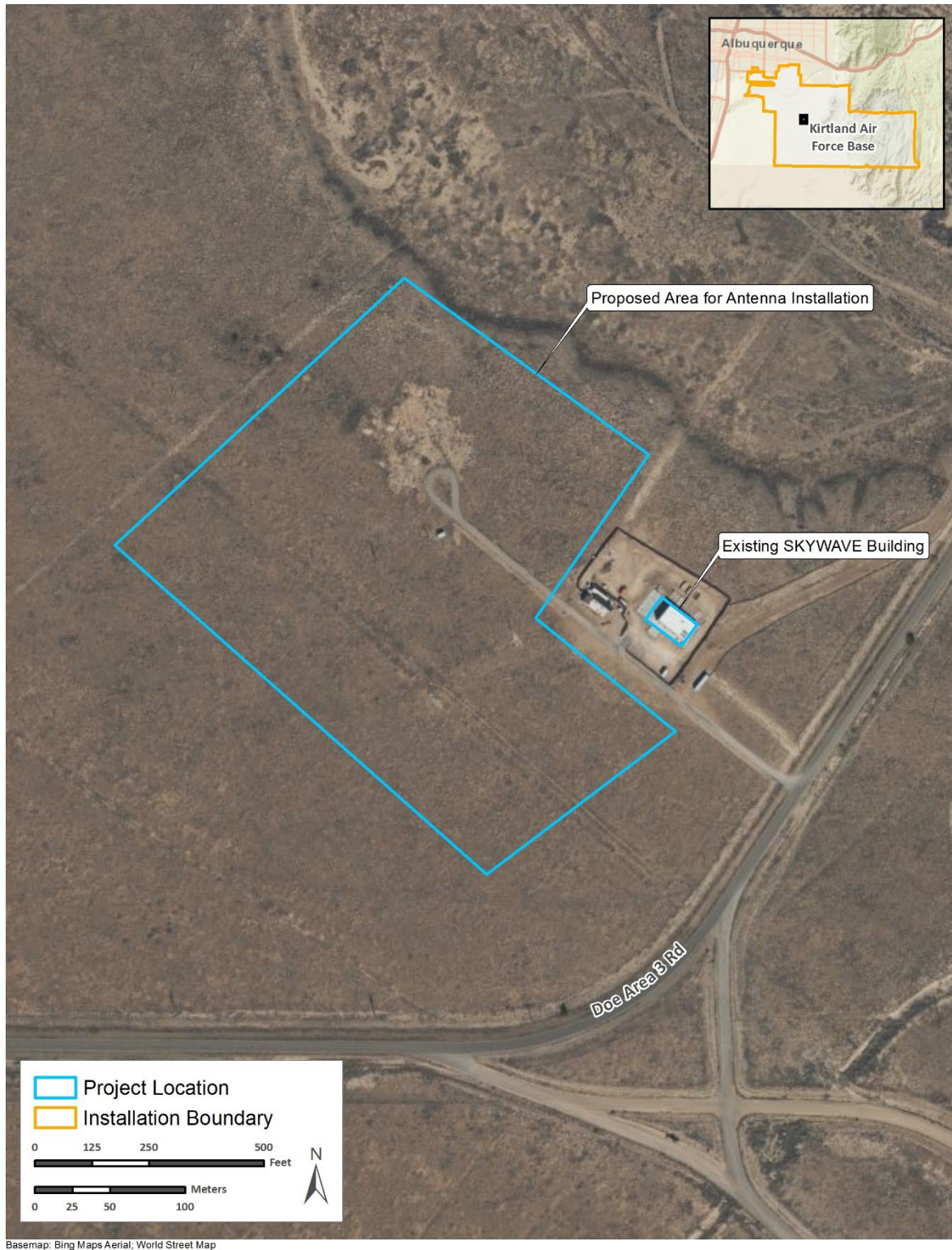
Figure 2-1. Proposed Area with No Known Utilities for Antenna Installations at SKYWAVE
