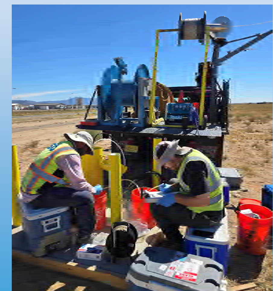
Groundwater Sampling of KAFB-WYO-6
