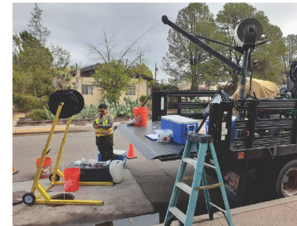
Collecting a groundwater sample with passive sampling
