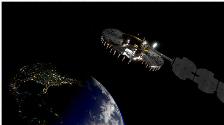
Artist's concept for NTS-3 in geostationary orbit. Harris Corporation will integrate NTS-3 using Northrop Grumman's ESPASat bus, building on EAGLE's flight heritage. Graphic credit: 1st Lt. Jacob Lutz, AFRL Space Vehicles
