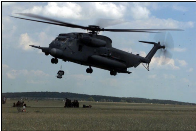
An MH-53J Pave Low III performs a hoist maneuver, 1998. Kirtland aircrews performed operational testing on the first Pave Low III prototype, as well as the aircraft's first search and rescue missions in 1980.
