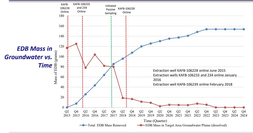
Pump and treat interim measure has achieved an estimated 95.8% reduction in the interim measure operational area of the dissolved EDB mass since 2016. EDB was not detected in Q4 2024, indicating no mass was removed during the quarter.
