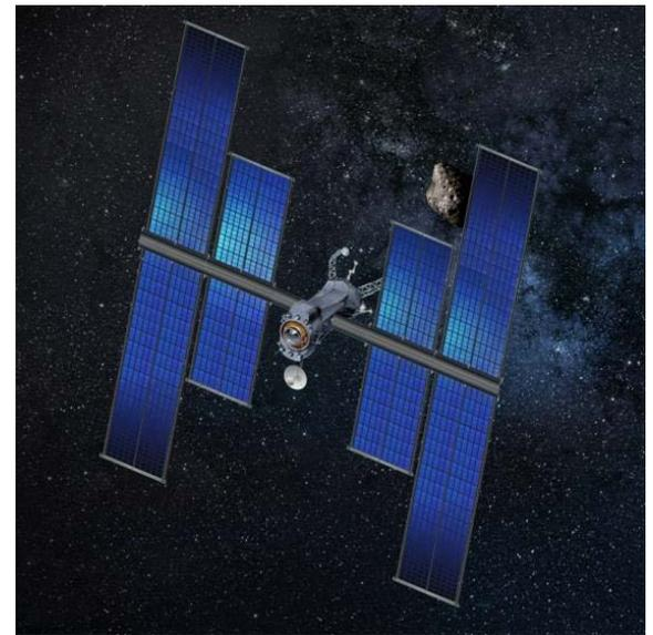
*Image of Space systems Loral 150 Kilowatt class solar electric propulsion vehicles with Roll-Out Solar Array.*
