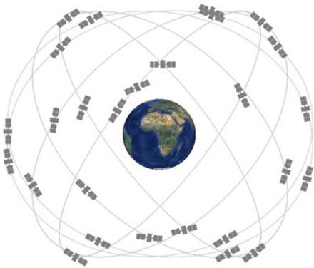
*Global Positioning System Constellation artist image. Satellites in the GPS constellation are arranged into six equally-spaced orbital planes surrounding the Earth*
