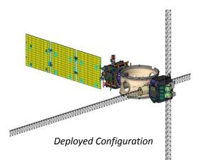
**Primary Experiment Payloads:** The **WPIx** will transmit and receive VLF waves in the 100 Hz to 750 kHz range in order to investigate their interactions with trapped electrons in the magnetosphere. DSX will also study the behavior of an insitu VLF antenna and characterize its farfield radiated patterns, as well as natural wave-particle interactions at MEO.
