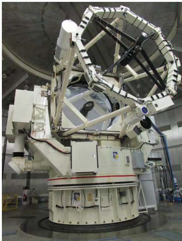
The 3.6-meter, 75-ton Advanced Electro-Optical System (AEOS) telescope shown above is the largest optical telescope in the Department of Defense. In addition the MSSS houses several other telescopes ranging from 0.4 to 1.6-meters.
